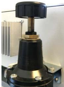
Figure 22: Pressure regulator for compressed air sweeping on the chamber rear, top right
